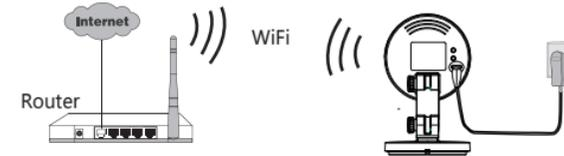
1. Connect the camera with power and wait for a moment, until the camera plays a sound "Hello, Foscam".
