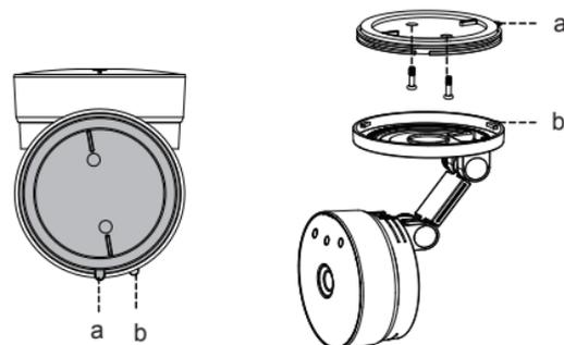
1. Rotate the base of the camera until points a and b are aligned, this allows for the mounting plate to be removed.
