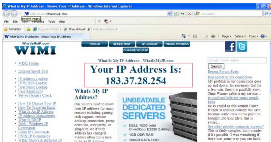
Figure 2.5 Get to know the WAN IP address of the router
