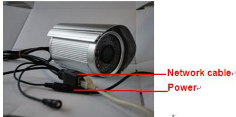
Figure 1.2 Plug the network cable and power
