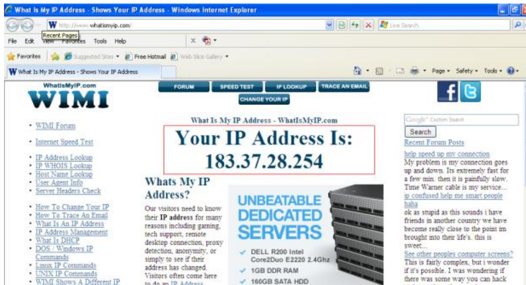
Figure 2.1 Get to know the WAN IP address of the router
